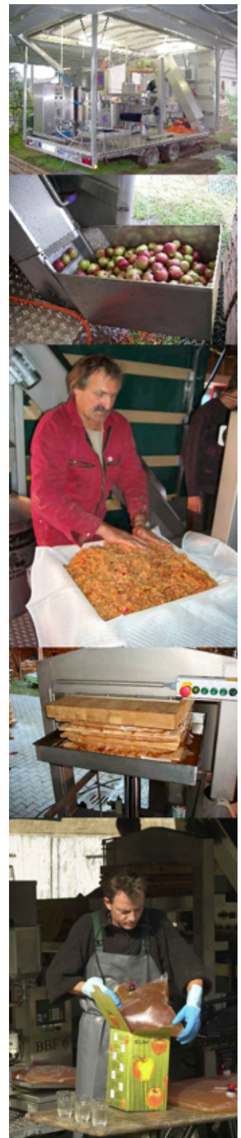
Mobile juicing and pasteurisation plant in Germany
