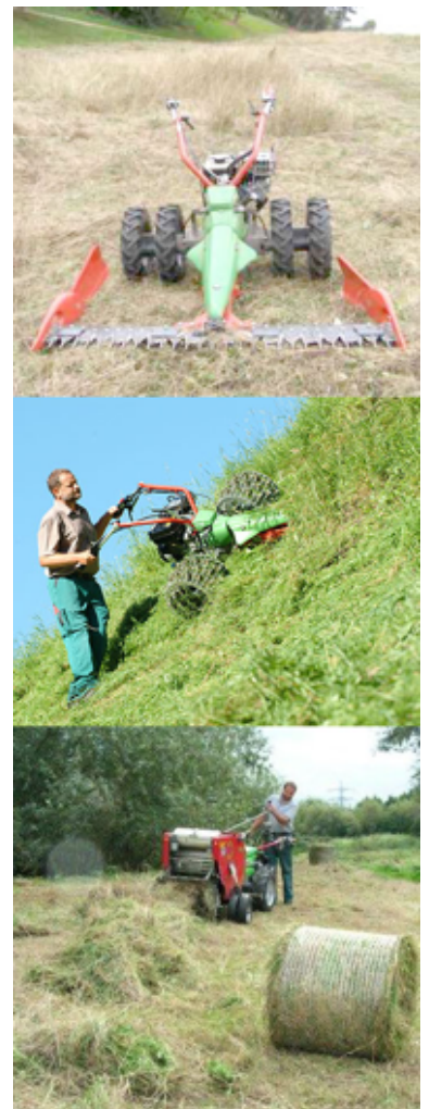
Modern finger bar mower with high output. Working on slopes. Small round baler.
